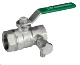
**EN** Chrome plated ball valve, female attacks, green lever handle and with drain cock. Standard port. 1/2"-3/4"-1": drain cock 1/4". 1"1/4-1"1/2-2 drain cock 3/8".
